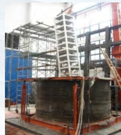
Shaking table test of soil structure interaction
