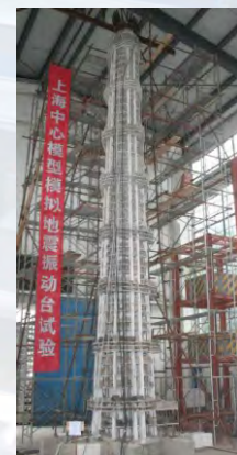
Shaking table test of Shanghai Tower
